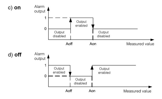
Fig. 9. Types of alarms: a) n-on; b) n-off; c) on; d) off.
