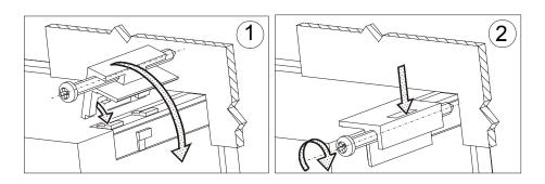
Fig. 2: Meter fitting
