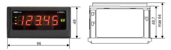
Fig. 3: Meter overall dimensions
